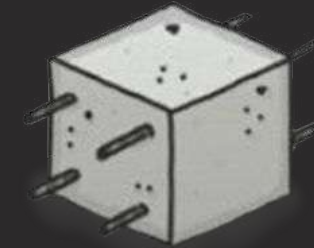
Reinforced concrete 635 kg CO 2 e / m 3 Ranges from 120 to 1 370 kg CO 2 e / m 3
