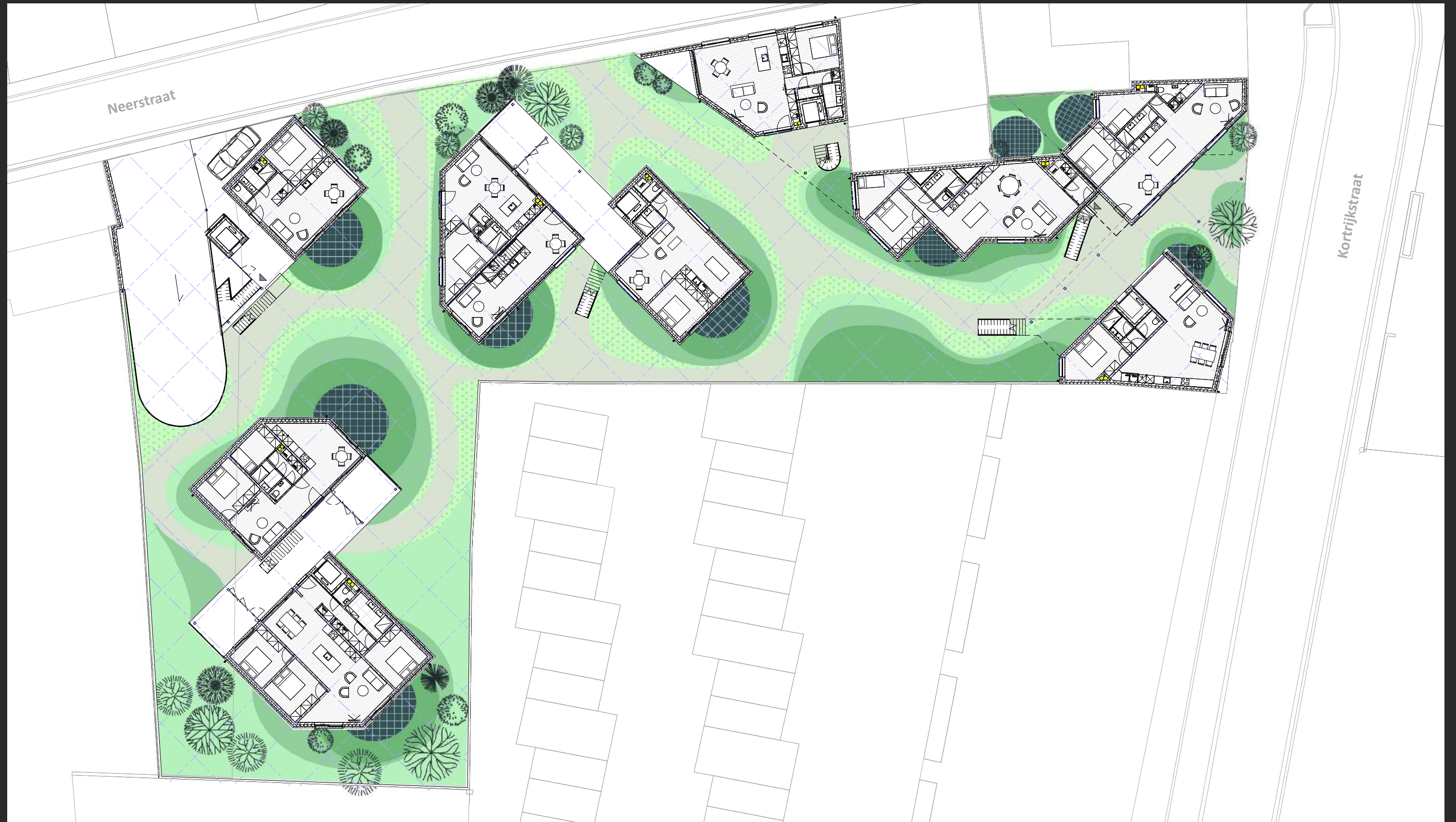
This is a masterplan where the same principle was developed and applied to a project for 36 housing units. The masterplan and the module are optimized for prefabrication.
