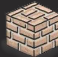
Clay brick wall 345 kg CO 2 e / m 3 Ranges from 260 to 1 100 kg CO 2 e / m 3
